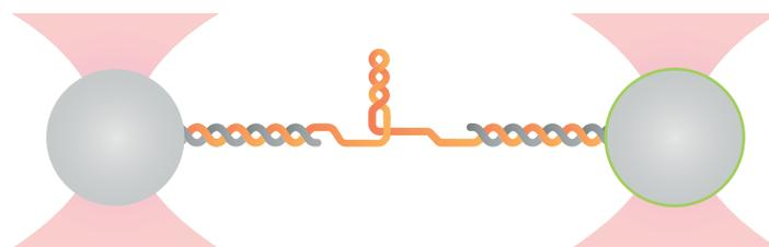
2 RNA hairpin structure tethered between optically-trapped beads via DNA/RNA hybrid handles. In order to ensure specific interactions with the coated beads, the handles are modified at their ends with the complementary interacting moiety to the beads.
