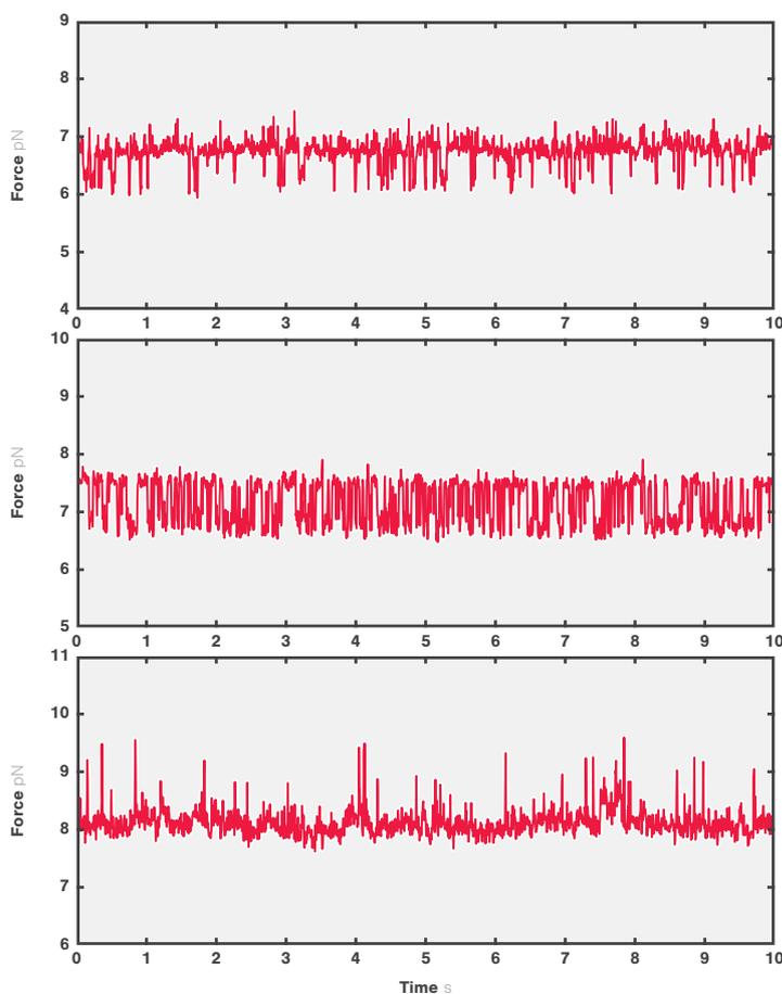
6 Ten seconds time traces at different initial values of tension 6.5, 7.5 and 8.2 pN. Points were decimated to 200 Hz from the high-resolution dataset collected at 50 kHz.
