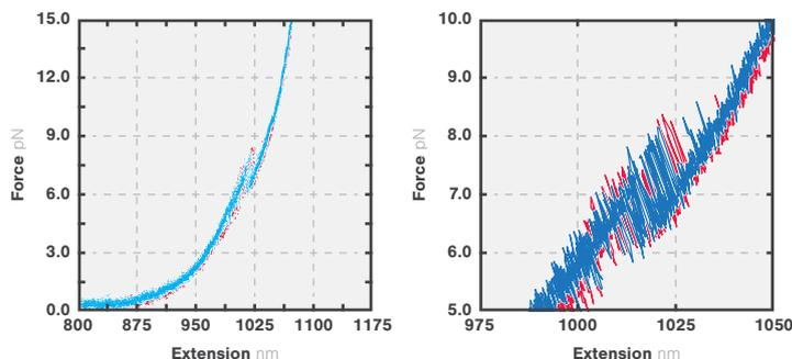
4 Force-distance curves corresponding to the extension (red, 10 nm/s) and retraction (blue, 10 nm/s) of a single RNA tether (left). Zoomed-in section of left image showing unfolding and refolding transitions (right). Data points were decimated to 200 Hz from the high-resolution dataset collected at 50 kHz.
