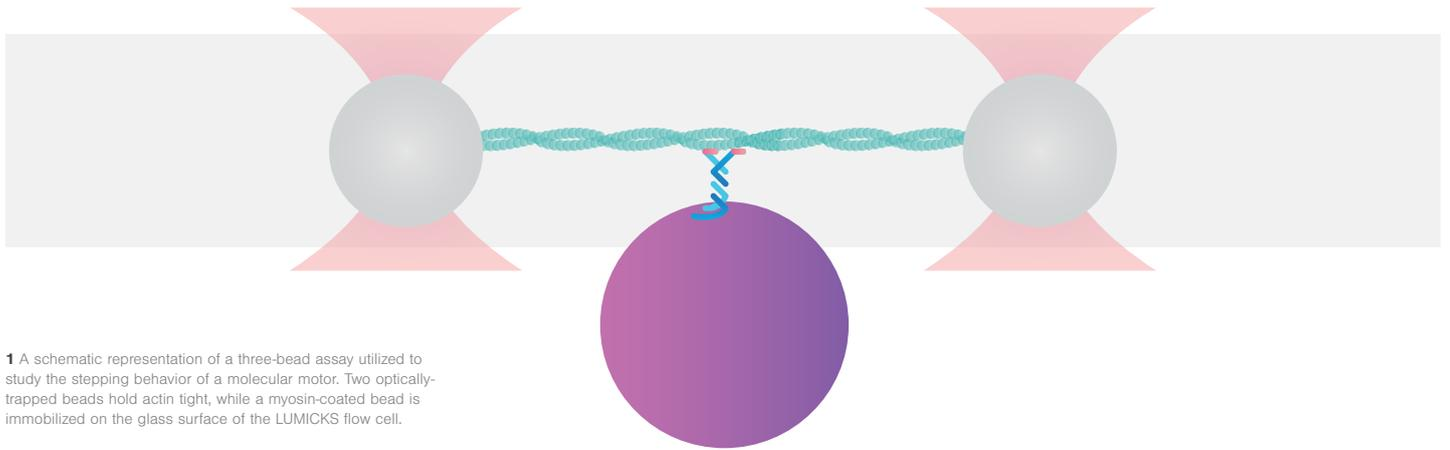
**1** A schematic representation of a three-bead assay utilized to study the stepping behavior of a molecular motor. Two optically-trapped beads hold actin tight, while a myosin-coated bead is immobilized on the glass surface of the LUMICKS flow cell.
