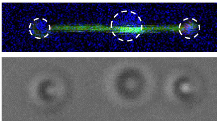
**2a** Fluorescent image (top) and brightfield image (bottom) of a single actin filament tethered between two trapped beads that has been brought into contact with a third bead, functionalized with myosin molecules (top).
